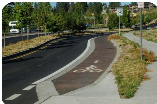
The photo above shows a raised bike lane with no parking. The bike lane is also done in a different colored asphalt to further distinguish it from the motor vehicle travel lane.
