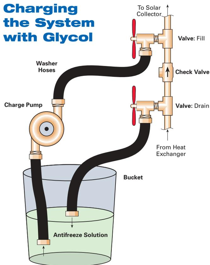
check valve, to anywhere in the bucket. You may need to elevate the bucket so that both hoses can reach it. The hose attached to the pump will need to reach the bottom of the bucket.
