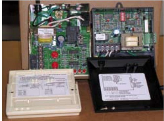
A Goldline GL-30 on the left and Heliotrope Delta-T on the right with the covers off. Note the diagrams and explanations on the covers.
