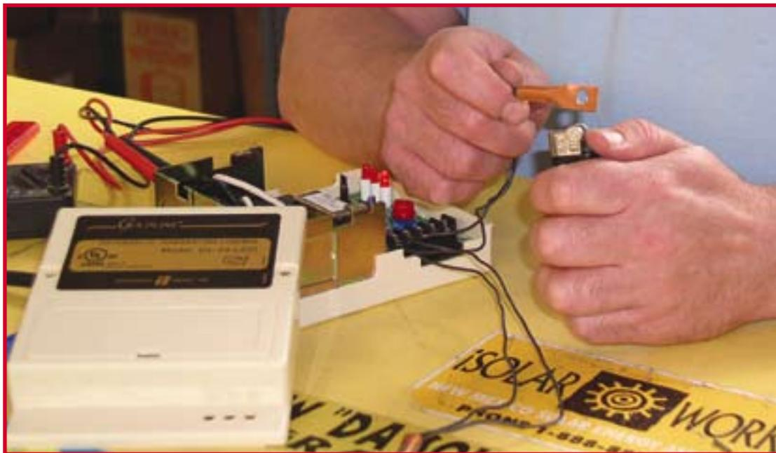
Smitty from AAA Solar uses a lighter to test a sensor connected to a Goldline GL-30 control.
