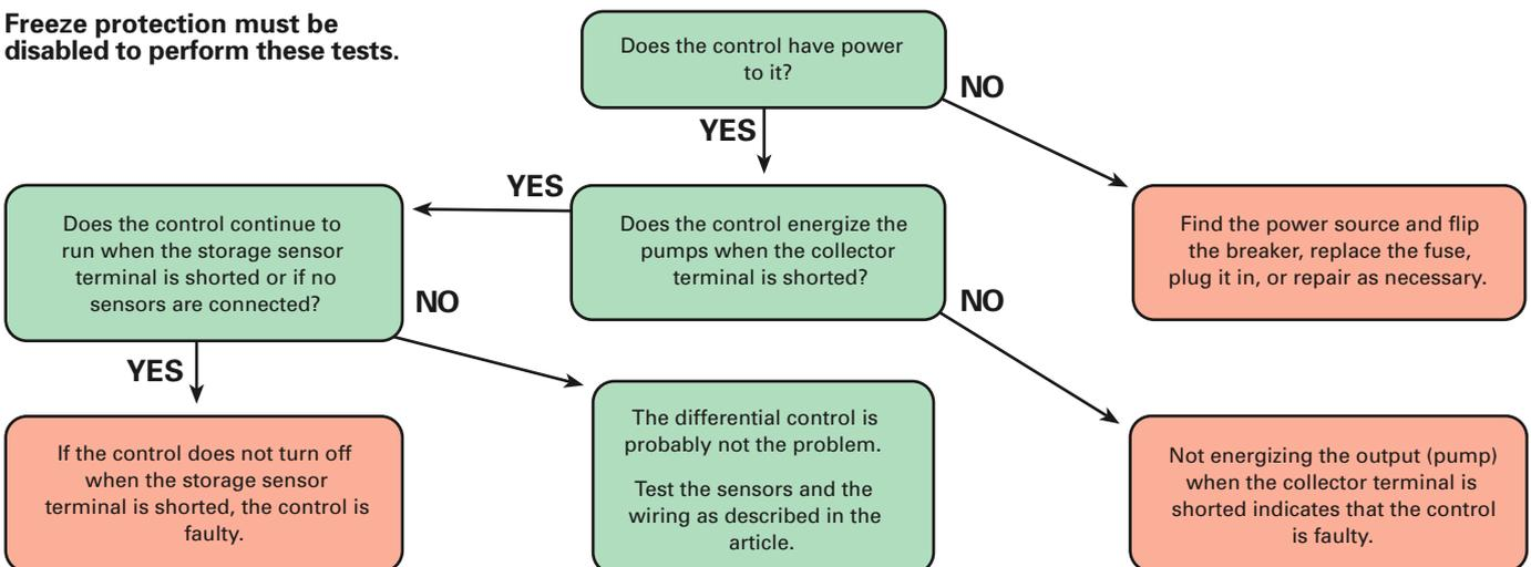
If the control does not energize the pumps when the collector sensor terminals are shorted, the control is bad. It will need repair or replacement, and with the rare exception of multiple problems at the same time, you have found the problem. Pat yourself on the back—troubleshooting is at the top of the pyramid in the world of field technicians.
