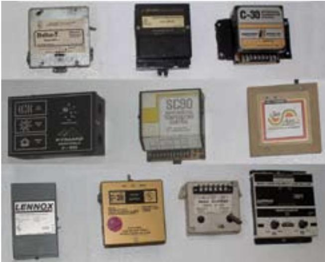
Ten differential controls used in solar water heating systems over the last 20 years.
