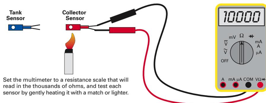
For one person to do the test at the end of the wires, the pumps will need to be able to be powered. If the control has an on-off-auto switch, they can be powered by flipping the switch to “on.” If not, they can be powered with an extension cord from another electrical receptacle. Set the multimeter for ohms, attach the probes to the collector sensor wires, and note the reading.
